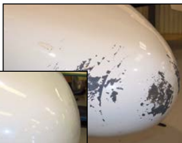
Above: Unretouched photo of eroded radome.
