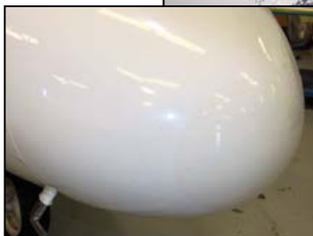
Above: Unretouched photo of eroded radome.
