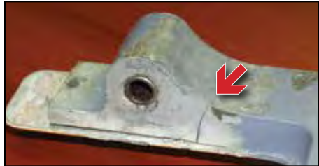
Original hinge showing stress fracture and cracking, separating casting from door skin.
