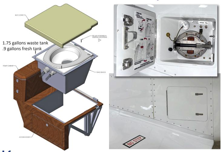
**CJ** series of aircraft. The original toilet is removed and replaced with a new flushing toilet designed to pump waste overboard through an industry standard external service panel. The new toilet is designed to fit into the existing toilet cabinet structure, requiring no changes to existing cabinetry or accessories.
