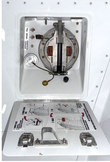
525B: Large Waste Valve Installation
