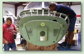
These highly experienced SkyWay sheetmetal techs are hard at work reconstructing a Citation nose section after it was damaged in a hangar collapse incident.
